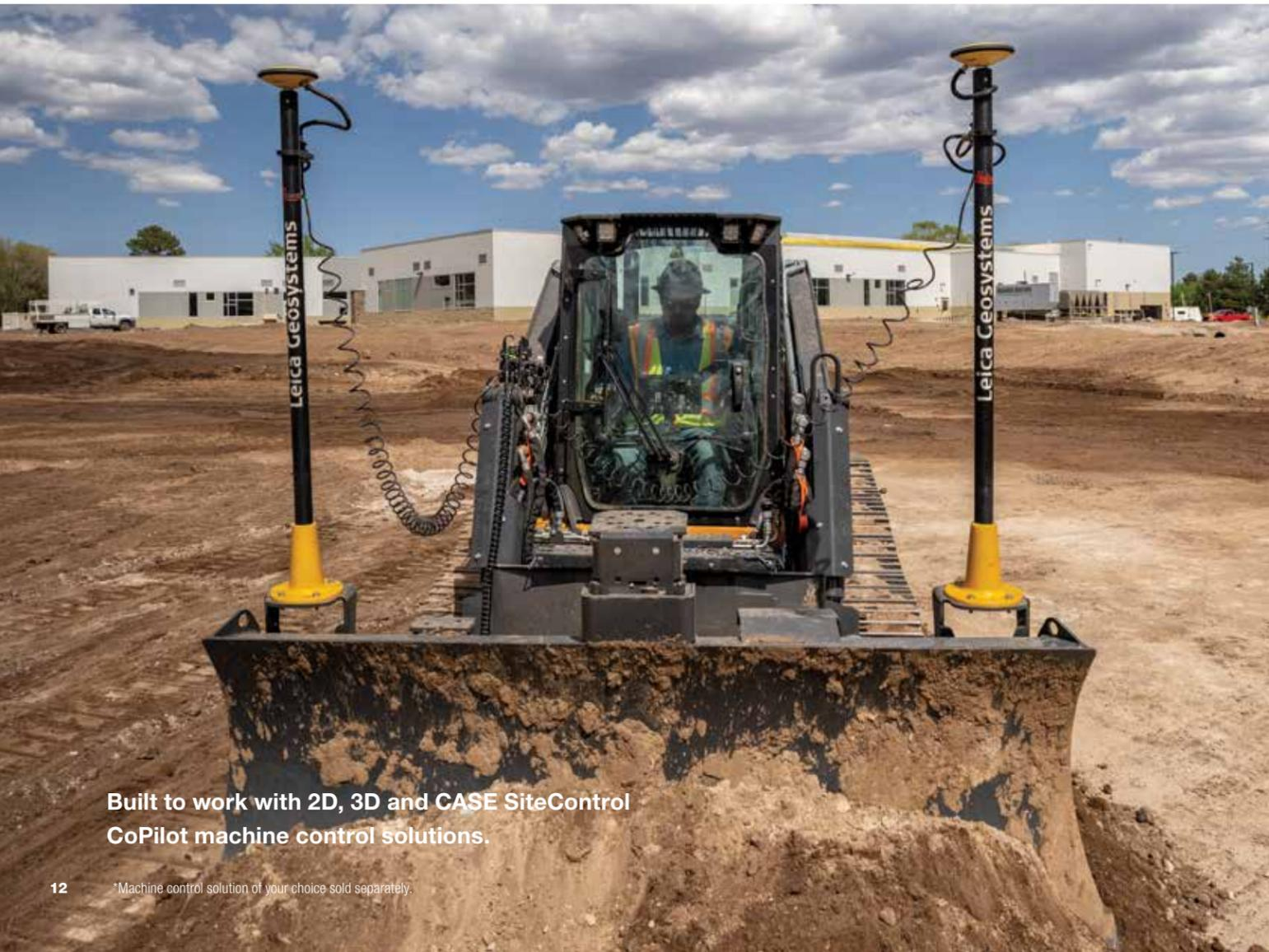
Built to work with 2D, 3D and CASE SiteControl CoPilot machine control solutions.
