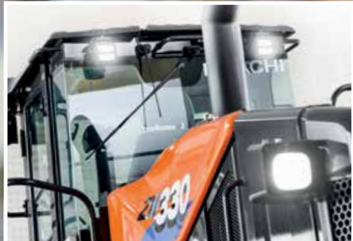
The standard LED work lights enhance visibility in low light conditions.
