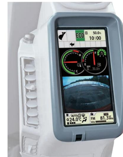
A multi-functional display provides key machine information, performance indicators, and on-board troubleshooting functionality with an integrated dial switch interface and 7-inch, high definition, color, multi-monitor screen. The display is fitted with an LED backlight to improve clarity and reduce reflective glare. 32 languages are provided for easier control and recognition.
