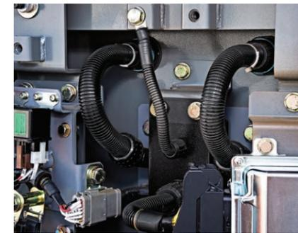
**SOLID CONDUIT WIRE HARNESSSES**
